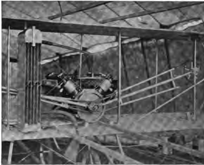
THE 60 HORSE-POWER MOTOR OF THE SMALL WRIGHT RACER, AND THE CHAIN DRIVE TO THE PROPELLERS
